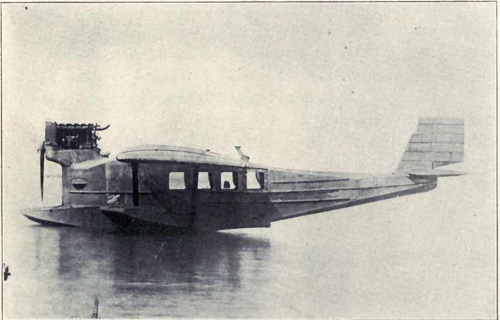
Zeppelin-Dornier "Dolphin" Monoplane All Metal Flying Boat Type DoCsII, 1921 Model. Carries six passengers besides pilot and mechanic. Speed 93 miles per hour, 185 horsepower motor. Gasoline consumption 11.9 gallons per hour. Weight empty 3200 pounds.
